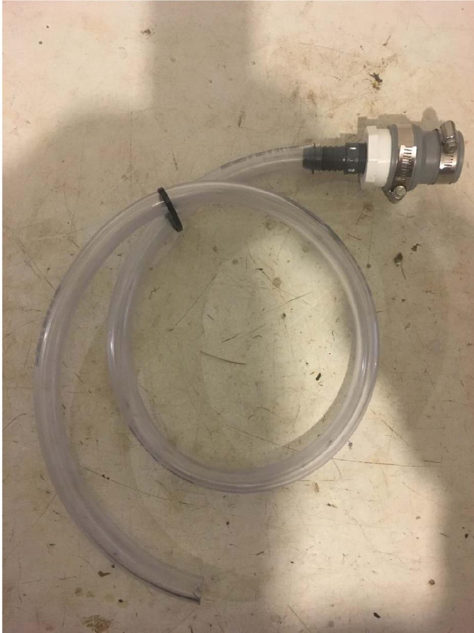
The final tubing is 3/4" ID with a threaded hose nipple with a threaded adapter and a rubber coupling to connect the boiler condensate discharge. This method is ideal for feeding directly into a condensate pump. It also allows for the removal of the hose when flushing.
